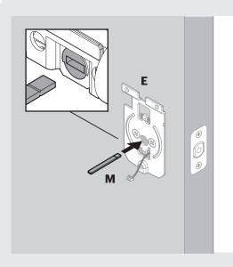
Align the colored edges of the connectors and ensure a tight cable connection.
