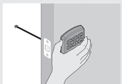
C Push the cable through the bottom hole.
