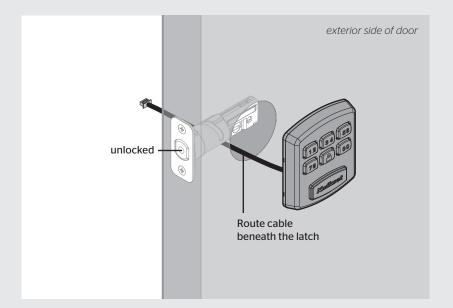
B IMPORTANT: Hold the exterior assembly on the outside firmly (or have a second pair of hands) for the next steps.
