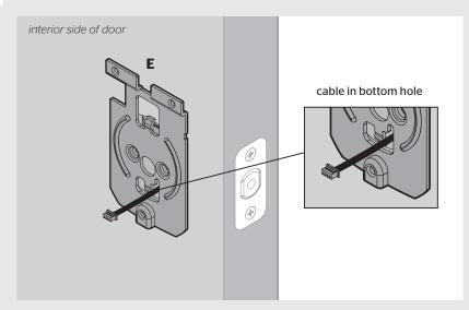
D Secure the mounting plate with the supplied screws.
